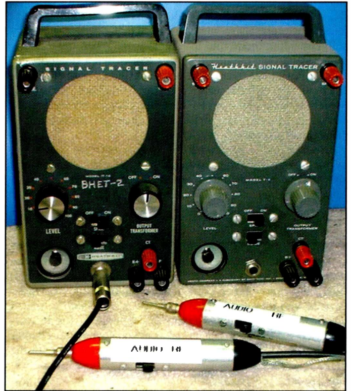
Photo A. The author's Heathkit signal tracers are a model T-4 and a model IT-12. They appear very similar on the outside and are identical internally. These two units were purchased as guinea pigs for this month's column.
