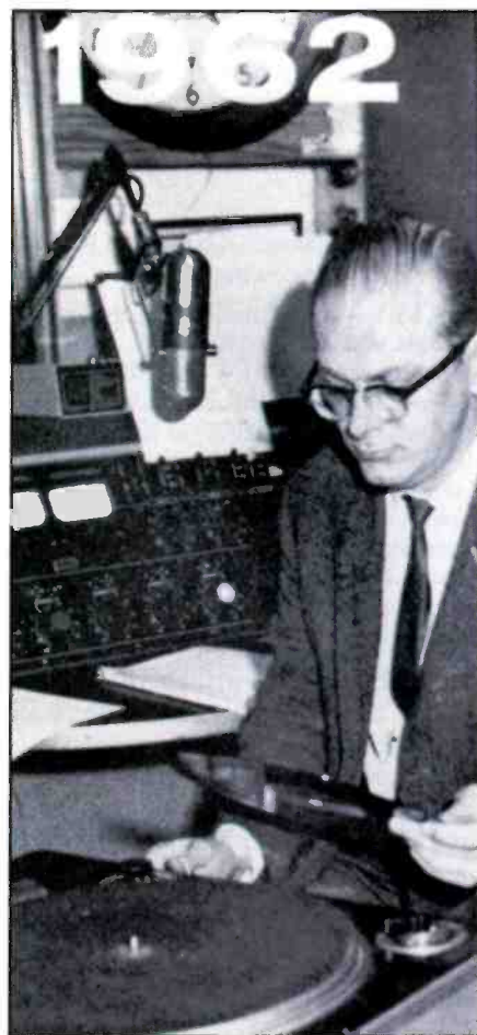
This "combo" operation—in which the on-air personality, not engineering department staff, ran the equipment—was pretty much the norm at most small-to-medium market radio outlets in 1962. Though KLZ 560 Denver offered the photo as evidence of its modernization, the 16-inch transcription turntable was then outdated and would have been a 12-inch model with recessed section for 45-rpm records if truly state-of-the-art in 1962.
