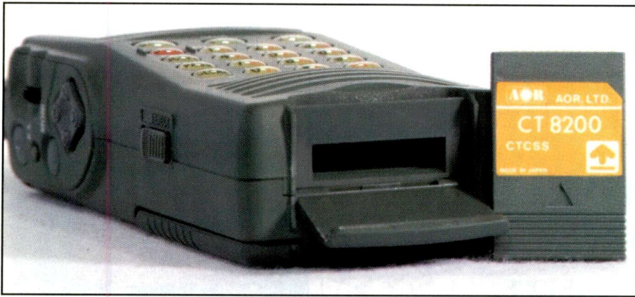
Many high-end receivers didn't include tone functions either. This AR-8200 required an add-on card, a unique approach that at least gave an option for those who needed the function for interference control.
