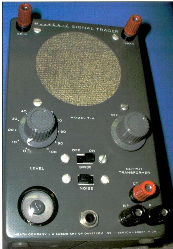
Photo B. Here's a nice close-up view of the control markings and front panel for the T-4 signal tracer. When picking out a unit, look for a front panel that's free of scratches and silk-screened lettering that's crisp and sharp. Any peeling or lifting paint might indicate a unit that has languished in a damp cellar for decades.
