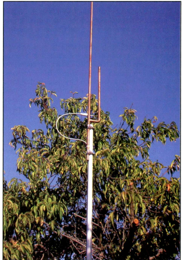
The KB9VBR J-Pole antenna at Laura's California QTH. (It's also a great scanner antenna; remember, it's tuned for 146 MHz, so if most of your local action is in the VHF band it'll perform quite well).
